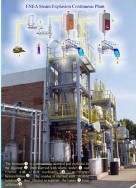
The biomass is continuously steamed and exploded in the digester. The steam is then filtered with water and filtered with a belt machinery. The residue is filtered with a solution. The residue is filtered with a solution. The residue is filtered to separate the lignin from cellulose.
